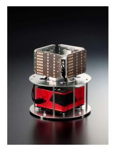
Hardware for which four miRadar8 modules are combined with NUC-PC.
