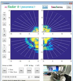
Evaluation software (Professional Version) is a Matlab execution file that controls coordinating operation for a maximum of four miRadar8 and displays processing results.
