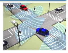
Connecting external trigger I/O signals enables multiple miRadars to operate in synchronization. miRadar1 is set to master mode because it does not have an external trigger signal input. miRadar2, 3, and 4 are set to slave mode, which operates in synchronization by an external trigger signal input.
